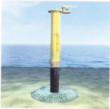
Monopile foundation with transition piece and scour protection. Flange height above
